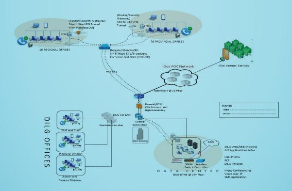
The LAN, WAN and IP Telephony aims to establish a data and voice infrastructure to the Central Office (CO) and three (3) pilot Regional Offices (ROs) that shall support the internal and external communication system. One of the major benefit of the department is the reduction of communication expenses by using local lines in the CO and establishment of voice connectivity to the ROs thru VoIP technology.
